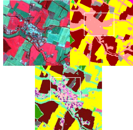
Figure 3: (a) Colored composition 08/07/10 Formosat (b) final classification (c) fusion with unsupervised classification to distinguish hedges and different stage of Built
